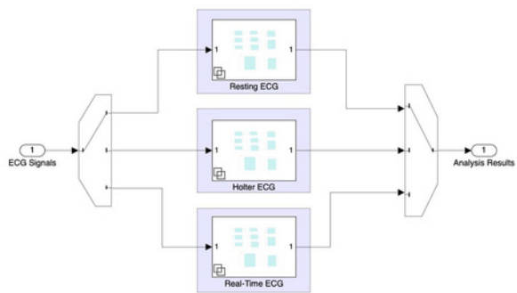
ECG signal analysis algorithms modeled in Simulink.
