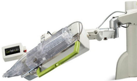
Corindus bedside unit with extended-reach arm and touchscreen.
